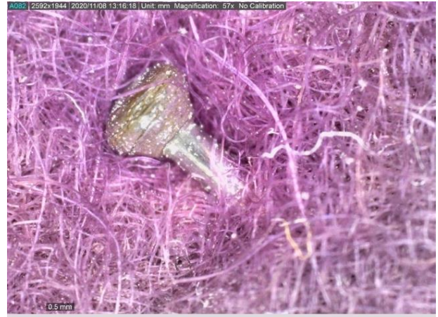
Detail of the hand made, wrapped pin head on an alleged broadcloth fragment of Napoleon's pall, magnification 57x ( TRC 2020.4528 ).
